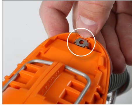
Klemme EU 869 aufstecken. Attach clamp EU 869 as shown.
