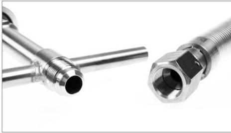
Check if connections correspond in type and size: LNG 13 vent coupling or Safety Break: 7/8"-14 SAE J512 45° male / female
