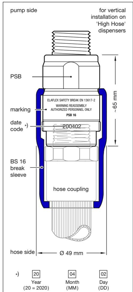
to **PSB** inlet. For NPT threads do not use Teflon tape but pipe sealant on threaded connections. Check the whole system for tightness.
