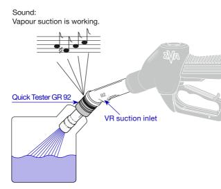
If there is no sound, the VR system may be defective. If in doubt, repeat the test with the spare Quick Tester to verify the result.
