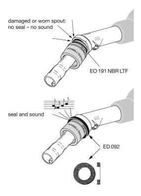
If the assembled O-Ring EO 191 NBR LTF has to be replaced, only use the original spare O-Ring which is included in the twin pack. This seal is electrically conductive and ensures electrical continuity between the tester and the nozzle.
