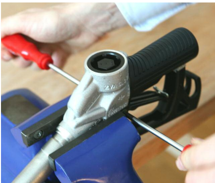
Unscrew front guard screws.
