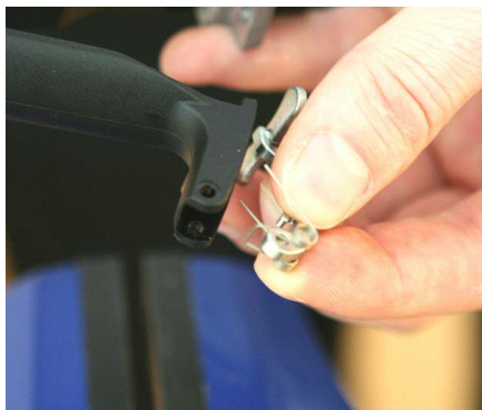
Remove hold-open latch and latch spring.
