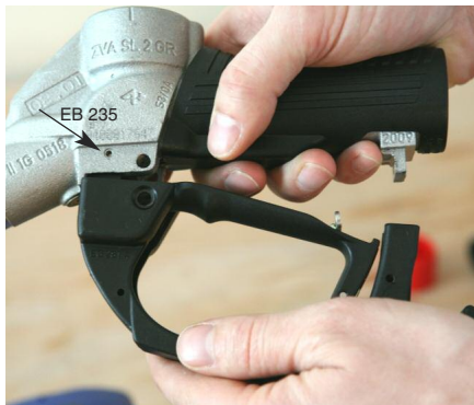
Remove guard. Pins EB 235 must not fall out.
