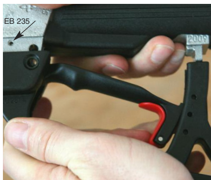
Control lever pins EB 235. Assemble guard.
