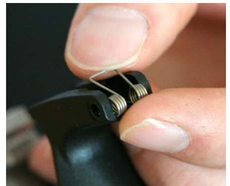
Re-insert latch spring in shown direction .
