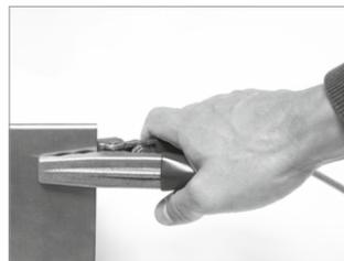
Connect the grounding cable from the station to the LNG tank or vehicle.
