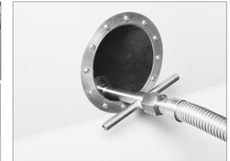
Put vent coupling back into dispenser coupling holder. Start refuelling. For operating instructions see manual of nozzle N-LNG.
