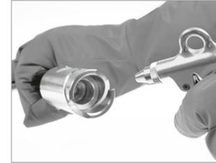
Now clean the vent coupling with compressed air. Completely remove moisture, ice and dirt before coupling the vent coupling to the valve seat. Check for visual damage, excessive wear and leakage.
