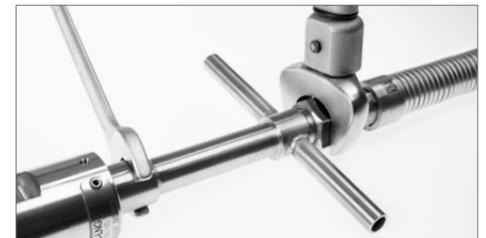
Connect the hose to the vent coupling. Torque to the hose fitting suppliers recommended tightening torque. Elaflex hose assemblies LNG 13: 60 Nm. **Do not use pliers.**
