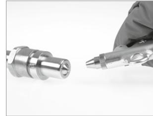
Clean valve seat with compressed air. Moisture, ice and dirt must be completely removed.
