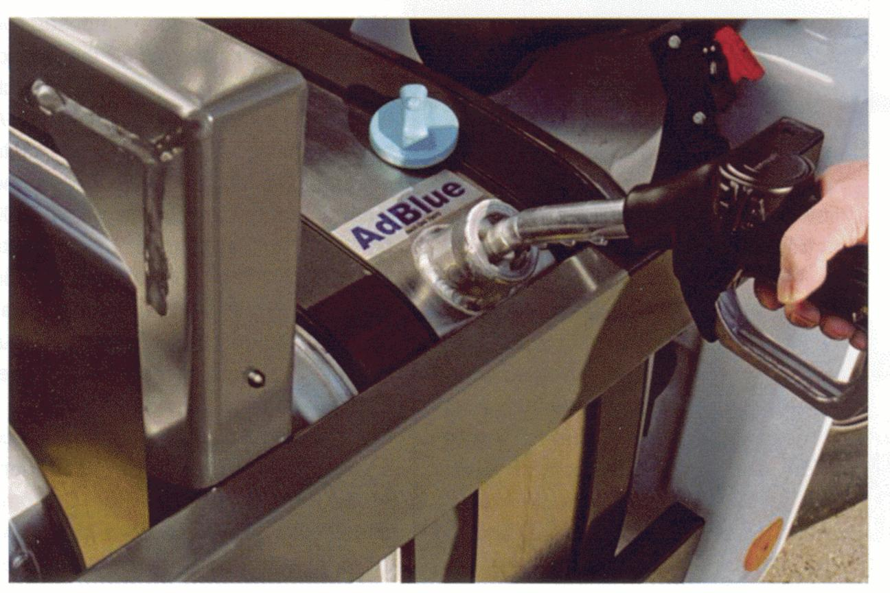
magnetic field. The blue "ELAFIX" magnet adapter is fitted in the filler neck of the AdBlue tank and provides the
