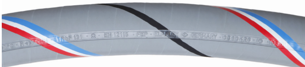
Example ELAFLO PLUS FEP - max. 10^6 Ohm resistance between hose end fittings - not conductive through the hose wall. According EN 12115 so far classified as M hose, according EN 12115 : 2011 now an \Omega hose.
