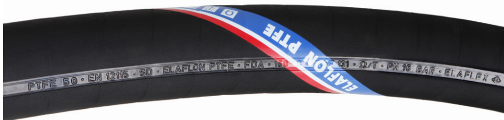
Example ELAFLO PTFE - max. 10^6 Ohm resistance between hose end fittings - max. 10^9 Ohm through the hose wall. According EN 12115 so far classified as \Omega hose, according EN 12115 : 2011 now an \Omega/T hose.
