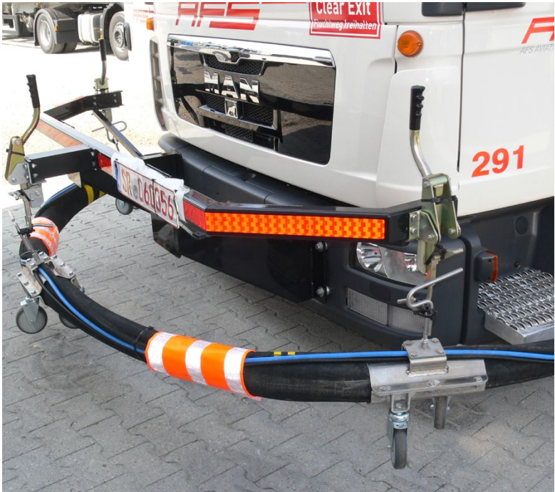
HD 100 C and HD 10 C / hydrant dispenser / the small hose serves as sensing line - Rohr, Germany
