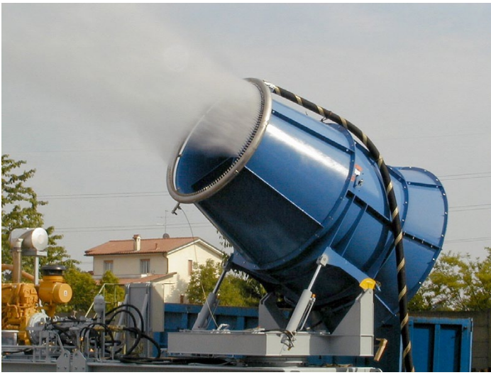
HD 100 Neon spiral / large aerosol canon to avoid dust spreading in mining and deconstruction - Ecology SRL, Italy
