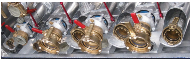
LTW hose assemblies / unloading road tankers at the petrol station / hoses stored lateral in the vehicle unloading hose size DN 100, vapour balance hose DN 50 - Schrader Beckum, Germany
