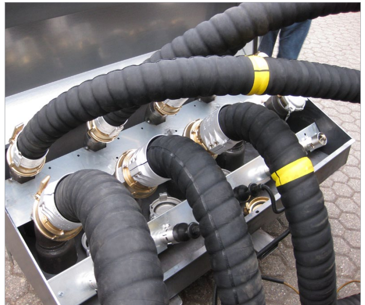
LTW hose assemblies / unloading road tankers at the petrol station / hoses stored lateral in the vehicle unloading hose size DN 100, vapour balance hose DN 50 - Schrader Beckum, Germany
