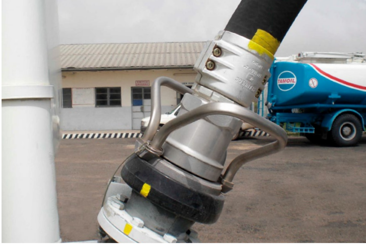
DDC-M 100 Dry Disconnect Coupling / large volume tanker loading or unloading - Tamoil, Eritrea
