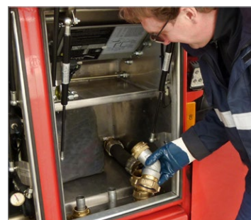
Paukner heating oil road tanker: adapter KR 50-2½" in the cabinet
