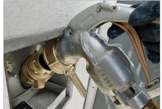
Narrow access: a connection of the nozzle to adapter 'TWÜ 13' is not possible
